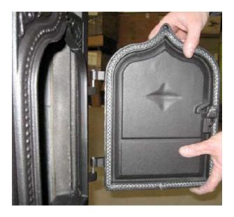
3. Lay the door face down on a suitable work surface. Use a putty knife or flat-head screwdriver to remove the old gasket. A wire brush can be used to clean out glue and old gasket residue from the gasket channel. Vacuum any leftover debris from the door and gasket channel.
