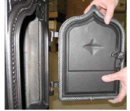
7. Close and open the door firmly several times to seat the gasket. If necessary, adjust the set screw on the door latch for the proper tension. Use a 7/16° wrench to loosen the lock nut and a 1/8° Allen wrench to turn the set screw.
